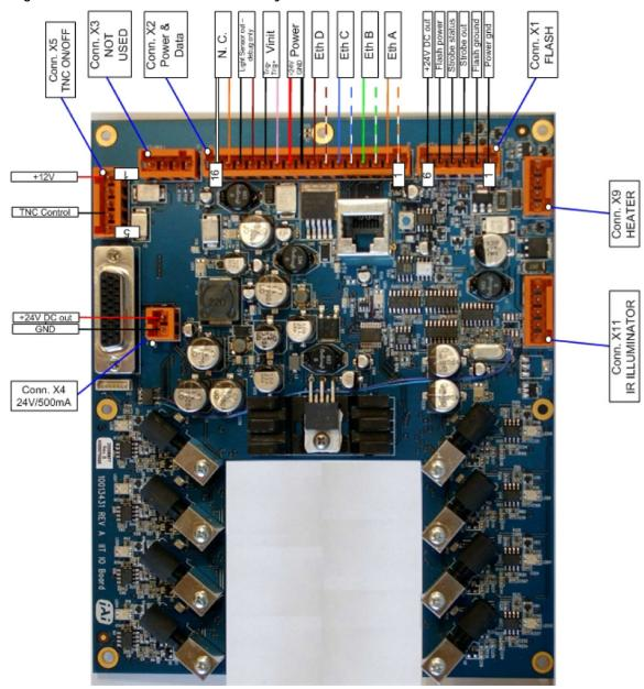
Figure 12. IIT I/O Board Power and Data Connector X2 signals
